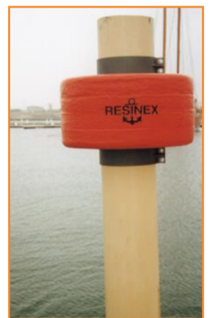
Pipe fender installed
