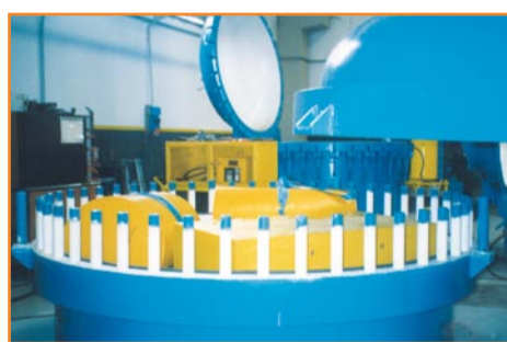
Pressure test for ROV modules at Adro Resinex Marine Research Centre
