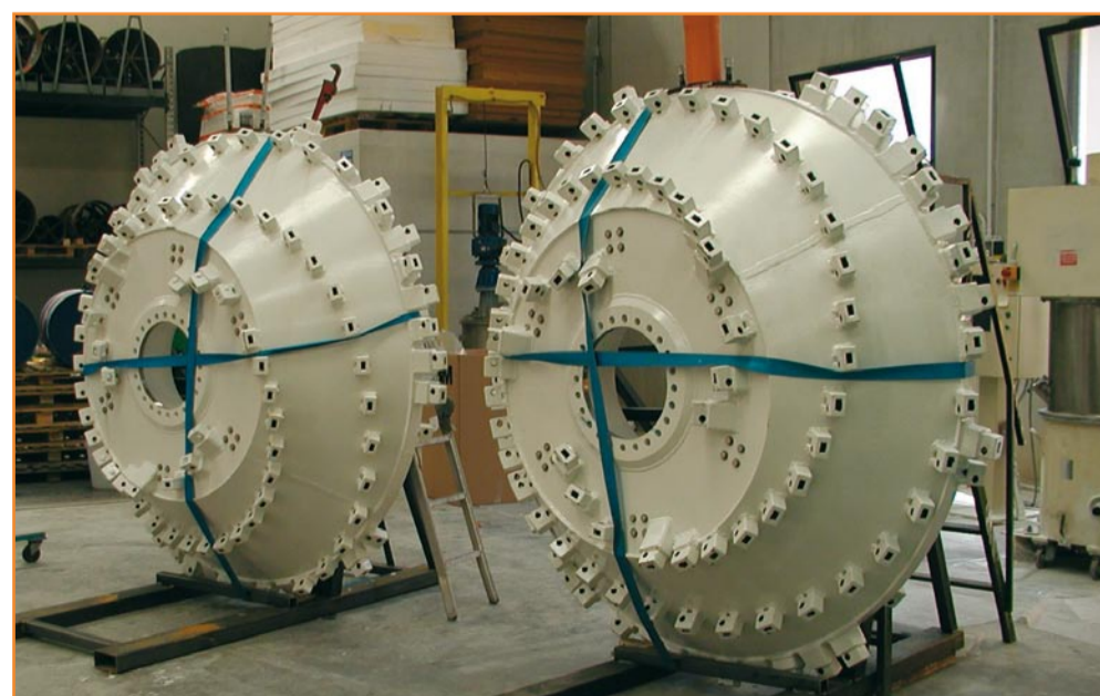
The excavation cutters during filling with Synt 3000
