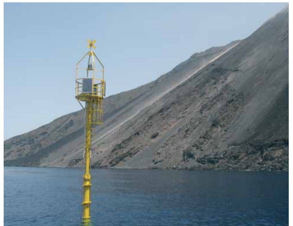
The beacon is equipped with many monitoring systems powered by solar panels.
