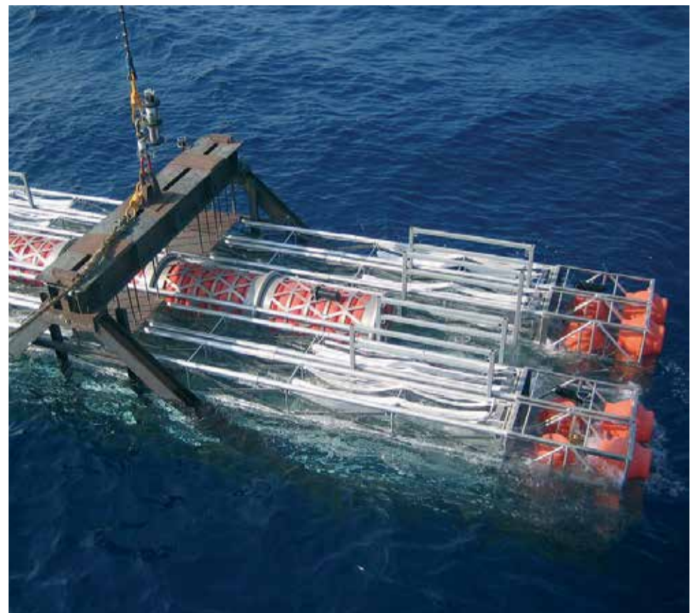
The Nemo module with by Resinex orange buoys 4000 meters water depth rated.
