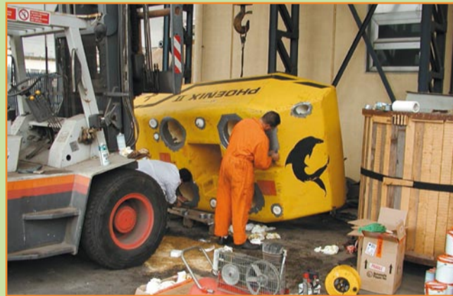
Renovation of ROV float
